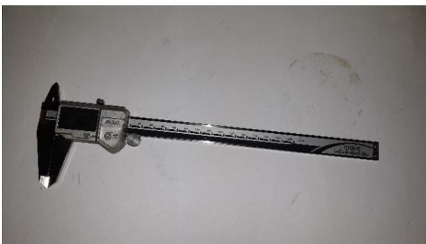
Gambar 4 Digital Vernier Caliper Mitutoyo
