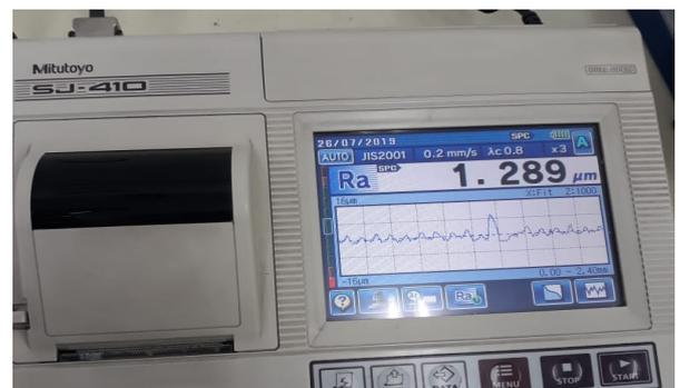
Gambar 5 Surface Roughness Tester Mitutoyo SJ-410
